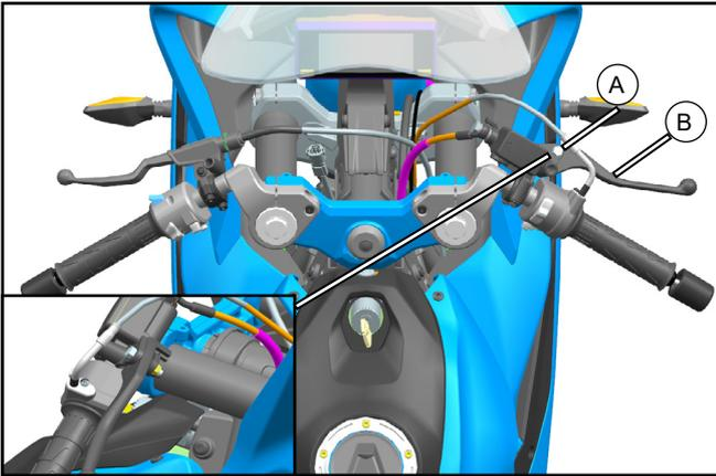
// Remove the bolt (A) and lever (B).
