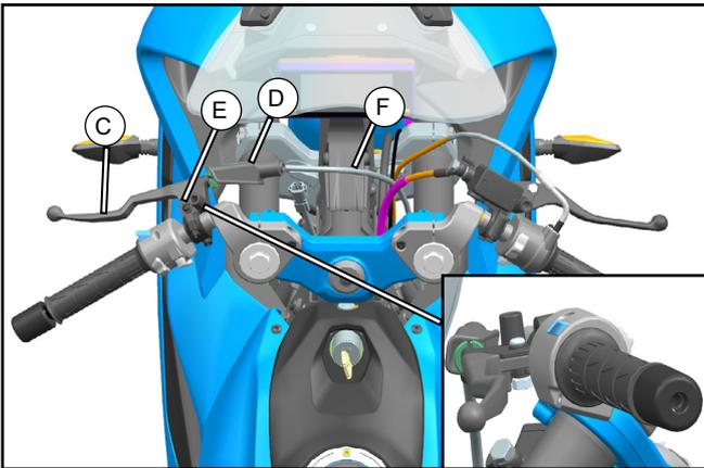
// Move the rubber dust cover (D) backward and remove the screw (E) and clutch cable (F) in turn. And finally remove the lever (C).
