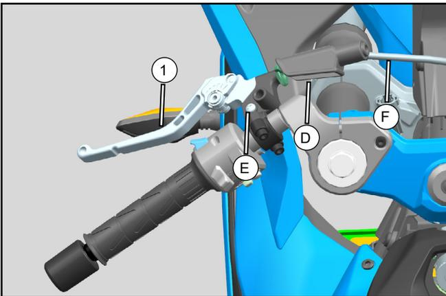
// Install clutch lever (1) with clutch cable (F) into original handle position, tighten with screw (E), and reset rubber dust cover (D).
